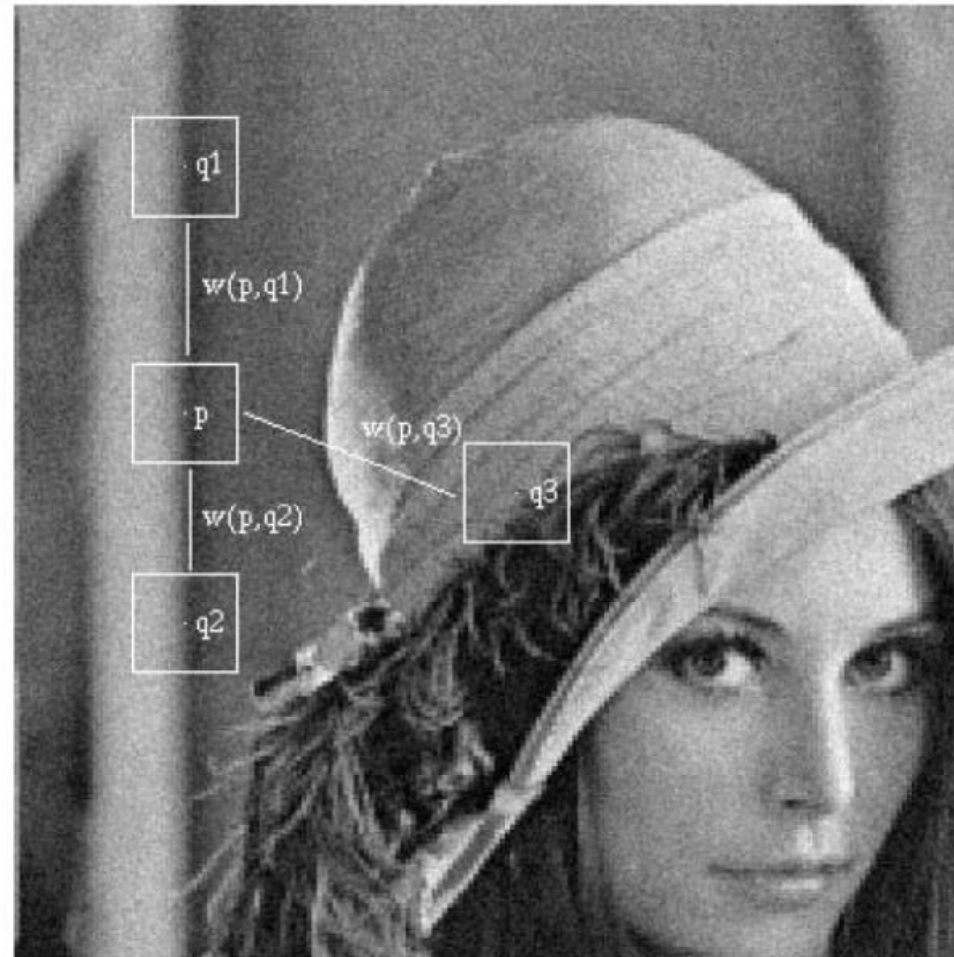
FIG. 6. q1 and q2 have a large weight because their similarity windows are similar to that of p . On the other side the weight w(p,q3) is much smaller because the intensity grey values in the similarity windows are very different.
